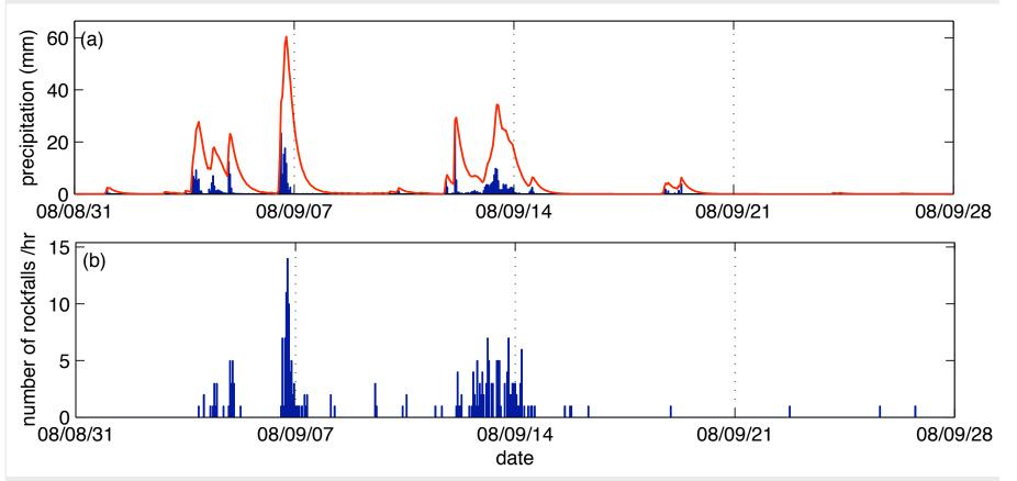
**Fig 8**: (a) hourly precipitation (blue) and antecedent rainfall  $P_c(t)$  (red), (b) number of rockfalls per hour.
